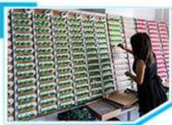
9. Aging test for travel charger
